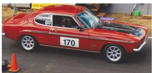
extractors inside coated and out. Sparco Seats, 5 speed Supra gearbox, electronic ignition, D port heads. Lightened flywheel and pressure plate, limited slip
